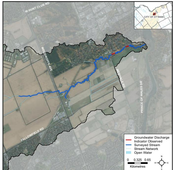
**Figure 27** Groundwater indicators observed in the Black Rapids Creek catchment.
