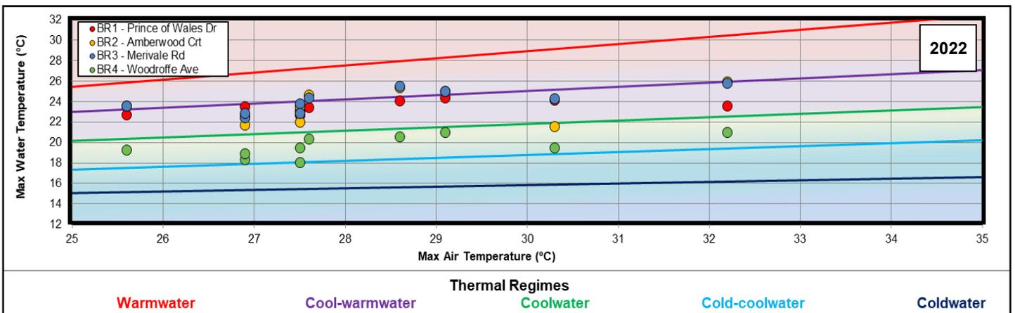
Figure 30 Thermal Classification for Black Rapids Creek with the five thermal regimes adapted from Stoneman and Jones (1996) by Chu et al. (2009): conditions range from **coolwater** (BR4) to the **cool-warmwater** (BR1-BR3) category for Black Rapids Creek in **2022**.
