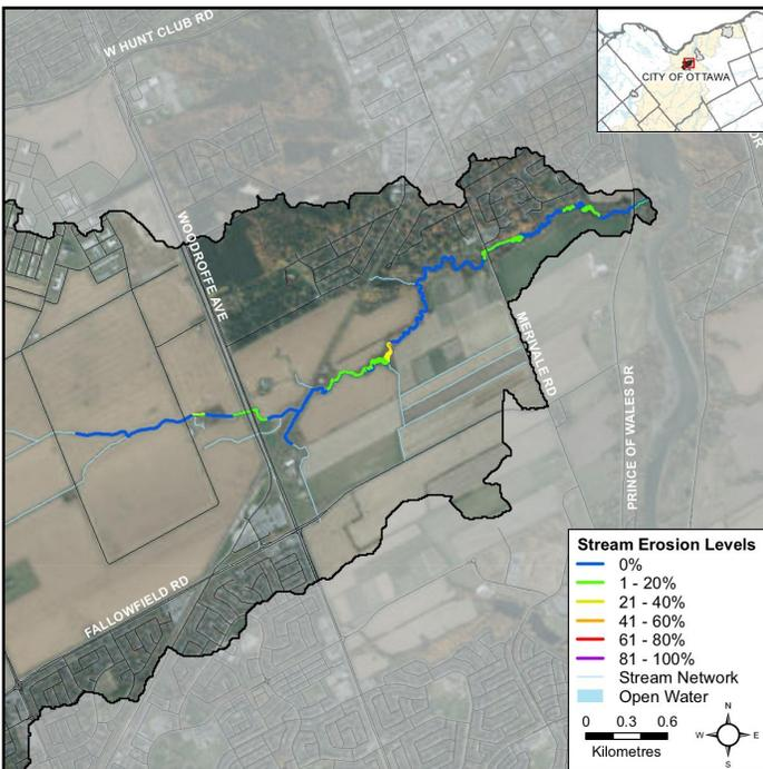
Figure 6 Erosion levels along Black Rapids Creek.
