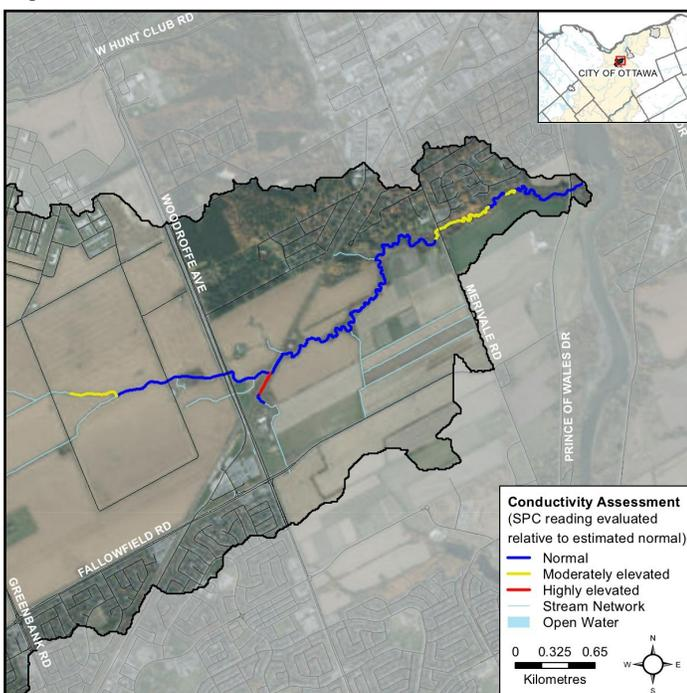
**Figure 26** Relative specific conductivity levels along Black Rapids Creek.
