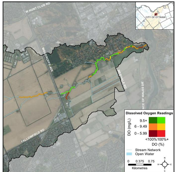
**Figure 25** Bivariate assessment of dissolved oxygen concentration (mg/L) and saturation (%) along Black Rapids Creek.
