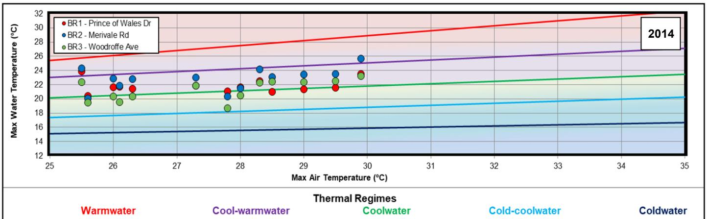
Figure 29 Thermal Classification for Black Rapids Creek with the five thermal regimes adapted from Stoneman and Jones (1996) by Chu et al. (2009): **cool-warmwater** category for Black Rapids Creek in **2014**.
