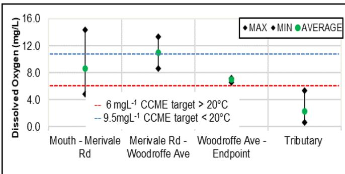
**Figure 22** Dissolved oxygen ranges along surveyed sections of Black Rapids Creek.
