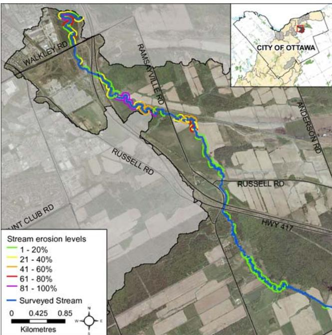
**Figure 4** Erosion along Ramsay Creek
