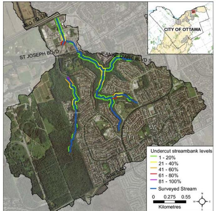
**Figure 5** Undercut stream banks along Voyageur Creek
