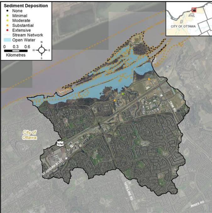
**Figure 38** Headwater feature sediment deposition in the Taylor Creek catchment
