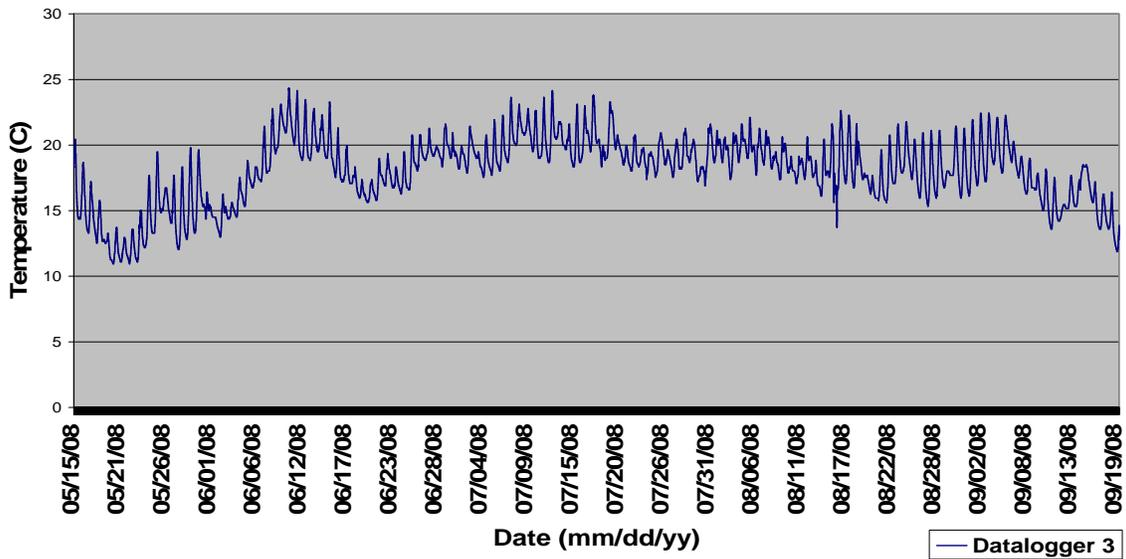
Figure 31. Temperature Profile for Datalogger 3 at Old Montreal Rd.
