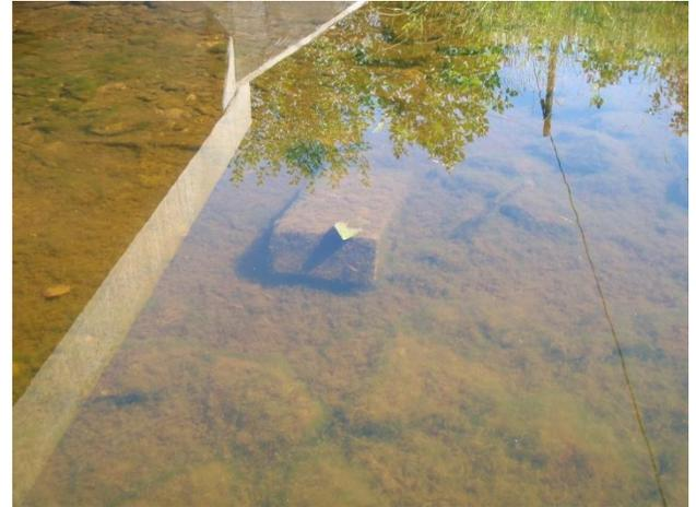
Photo of datalogger deployed in Stevens Creek on a block
