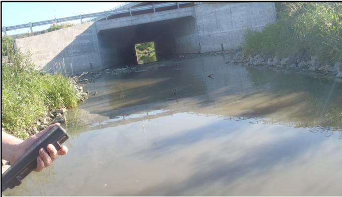
Collecting water chemistry measurements with a YSI probe on McEwan Creek
