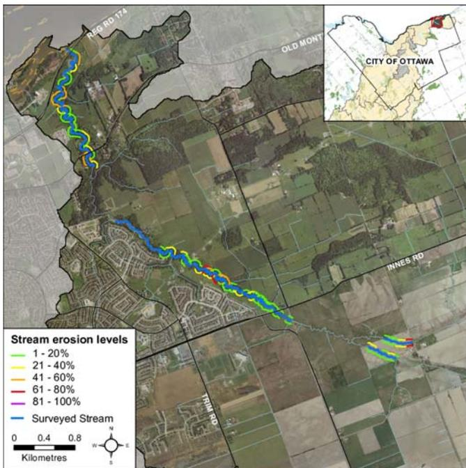
**Figure 4** Erosion along Cardinal Creek
