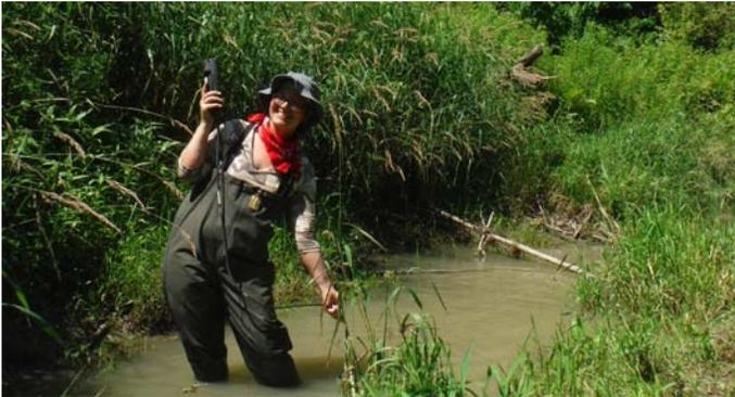
A volunteer collecting water chemistry measurements with a multiparameter YSI probe on Becketts Creek
