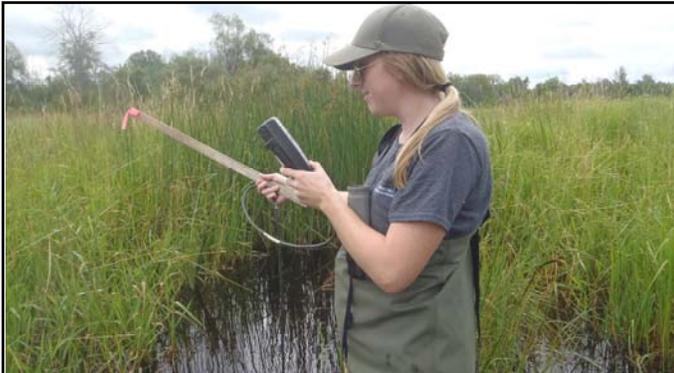
Collecting water chemistry measurements with a YSI probe along the Ottawa West Tributary 1
