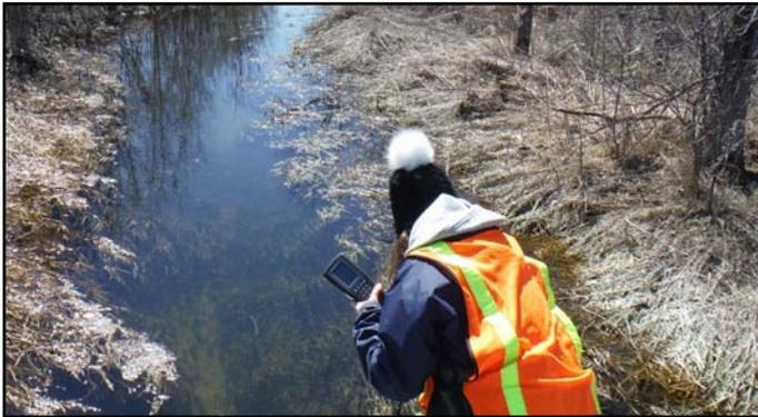
Collecting water chemistry measurements with a YSI probe in the Stevens Creek catchment
