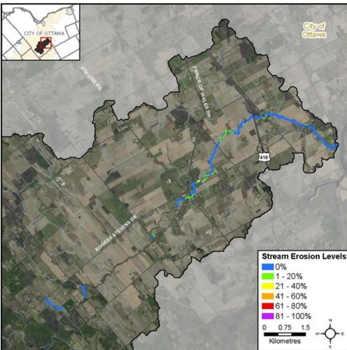
Figure 6 Erosion levels along Stevens Creek
