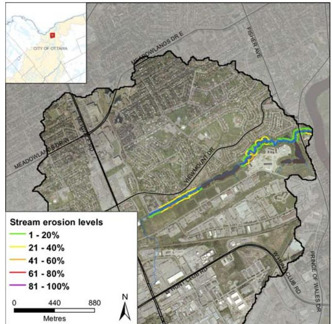
Figure 4. Erosion along Nepean Creek
