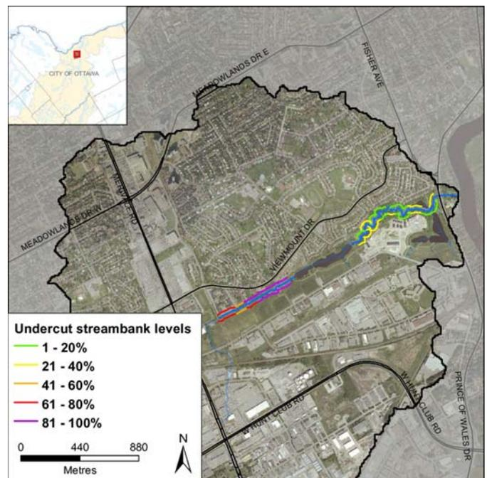
Figure 5. Undercut streambanks along Nepean Creek
