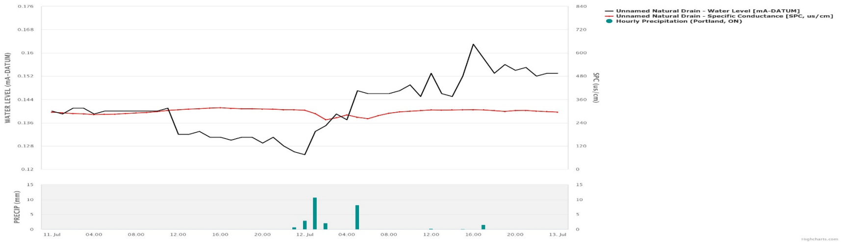
Figure 56. Analyzed specific conductance (SPC, uS/CM) and water level (m above datum) collected from a deployed solinst LTC logger deployed in an unnamed natural drainage feature located adjacent to the Portland Bay Conservation Area in Portland, ON compared to hourly precipitation data collected from RVCA's Portland Rain Gauge for the time period of July 11 th to 13 th , 2022.
