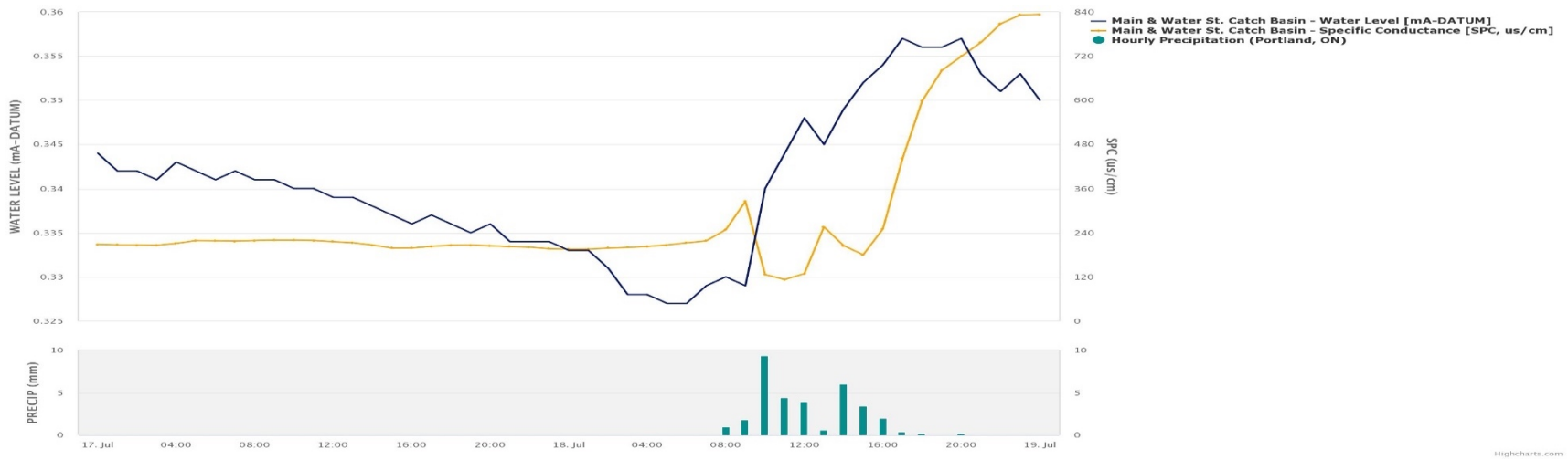
Figure 8. Analyzed specific conductance (SPC, uS/cm) and water level (m above datum) collected from a deployed solinst LTC logger deployed within the Main St. & Water St. catch basin located in Portland, ON compared to hourly precipitation data collected from the RVCA Portland rain gauge for the time period of July 11 th , 2022, to July 13 th , 2022
